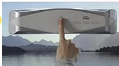
Ford revealed a prototype technology, called Feel the View, that allows the blind passengers to "feel" what they can't see outside a car's window. The automaker released a video this week touting the technology. Here's how it works: A camera attaches to the car's window and takes...
